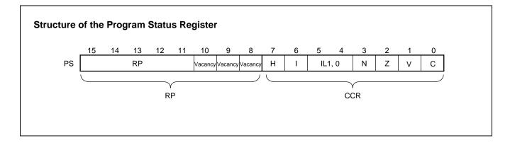
The RP indicates the address of the register bank currently in use. The relationship between the pointer contents and the actual address is based on the conversion rule illustrated below.
