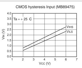
V<sub>IHS</sub> : Threshold when input voltage in hysteresis characteristics is set to "H" level. V<sub>ILS</sub> : Threshold when input voltage in hysteresis
